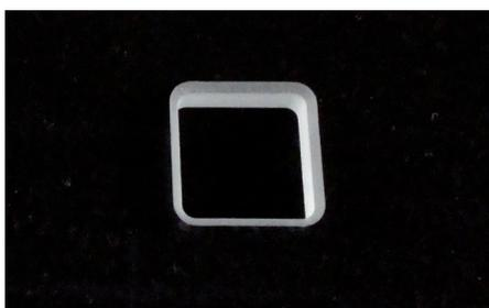
Bevelled LASER drilling
