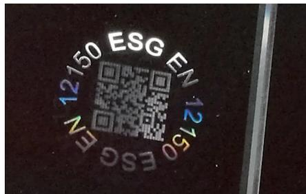
Hi-res LASER marking on tempered glass
